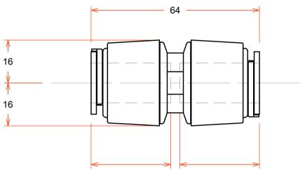
Pipe Insertion Depth: 30mm Pipe Insertion Depth: 30mm
